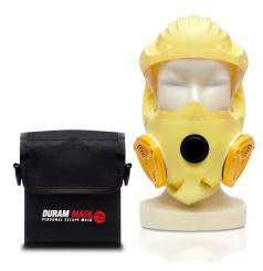
A certified personal respiratory protective device intended for evacuation in emergency situations involving smoke and hazardous fumes. The COGO provides users with short-term respiratory protection against smoke and Carbon Monoxide inhalation, and is tested against CO, HCl, HCN and Propenal. The COGO is certified under European Standard EN-403, and holds the EU CE mark.
